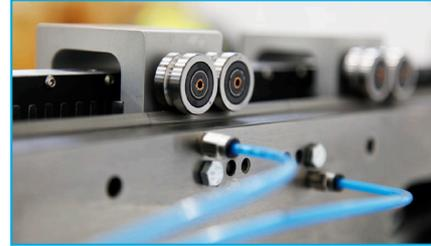
It is highly recommended that lubrication ports are situated once every 3 meters of track for systems without lubricators, or once every 6 meters of track for systems with lubricators.
